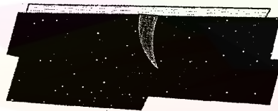
Step 3: Developer powder applied to draw penetrant out of crack
